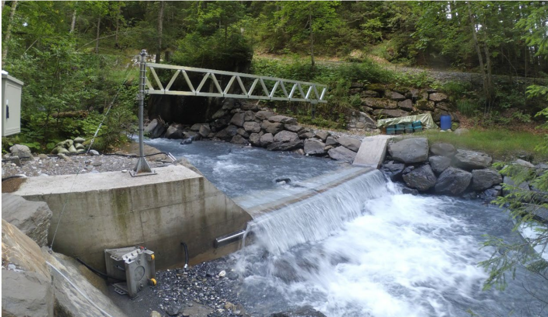
Figure S2. Automatic picture of the Avançon de Nant measurement station at the Vallon de Nant outlet on July 30 th 2018. The river stage measure by the SONAR above the middle point of the river is disturbed upstream by a rock.
